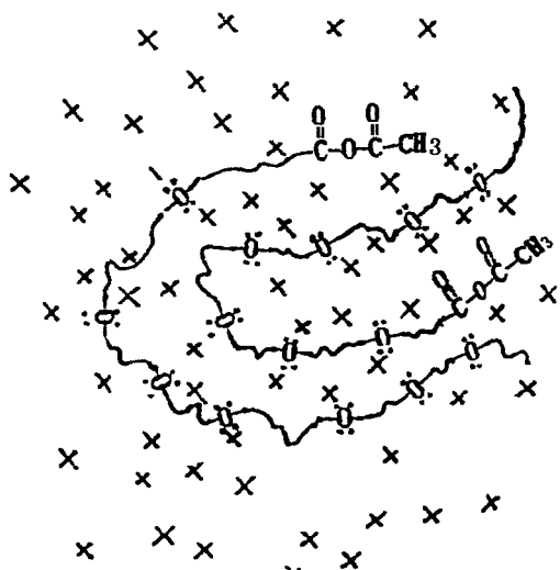
Figure 6 Sketch of the electrostatic shield of polyether segments to carbonyl carbon.
